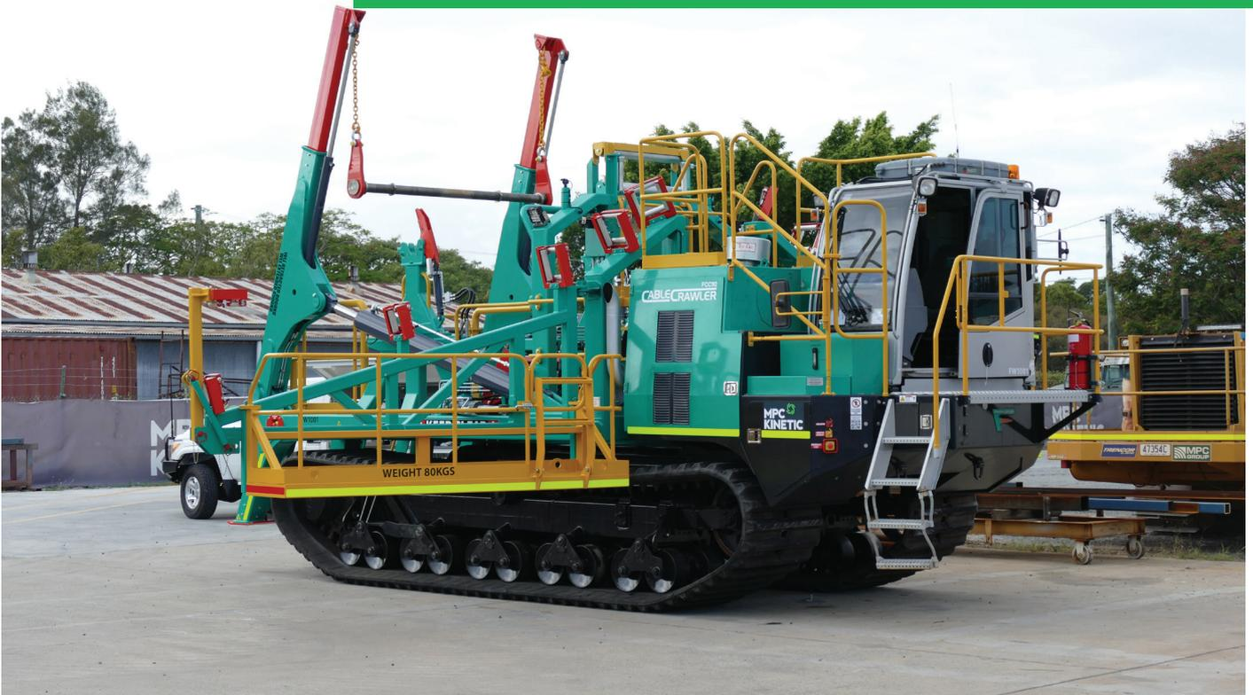
MPC Kinetic's innovative cable crawler is the fastest and safest method for installing High Voltage and Fibre Optic cable within the industry. The purpose-built machine provides clients with a cost-effective and safer solution for installing cables up to 110mm in diameter.
